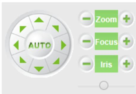
**PTZ Control:** To use eight directional keys to change the image orientation or click on the “AUTO” button to allow auto-rotation.
