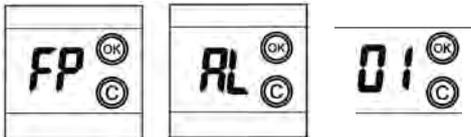
If "FP" is selected, Press **OK** key, then place the registered finger twice on the sensor or input the password twice or swipe card twice to delete the fingerprint or password or card. Press **OK** key to continue delete other users or press **C** key to exit delete status.
