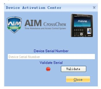
Input the Device Serial Number of Device.Click "Validate" Tab to continue(The red point will turn green when the validation is successful.):
