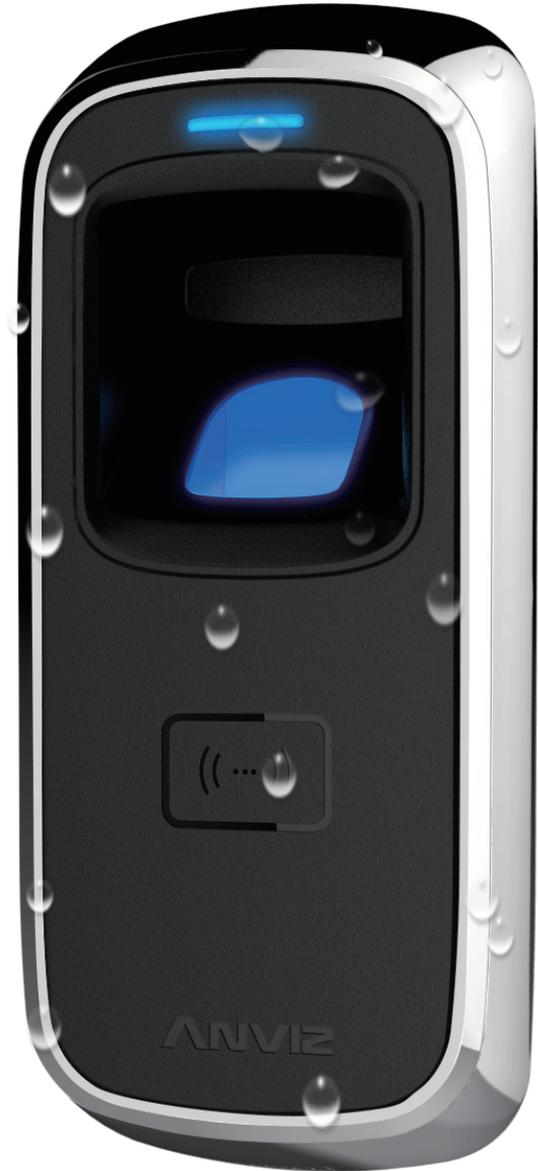
M5 by ANVIZ is a compact access control device that is designed to fit most door frames. A metal casing, with IP65 water-proof design, makes it suitable for indoor or outdoor applications. M5 supports 125kHz proximity cards and fingerprint identification.
